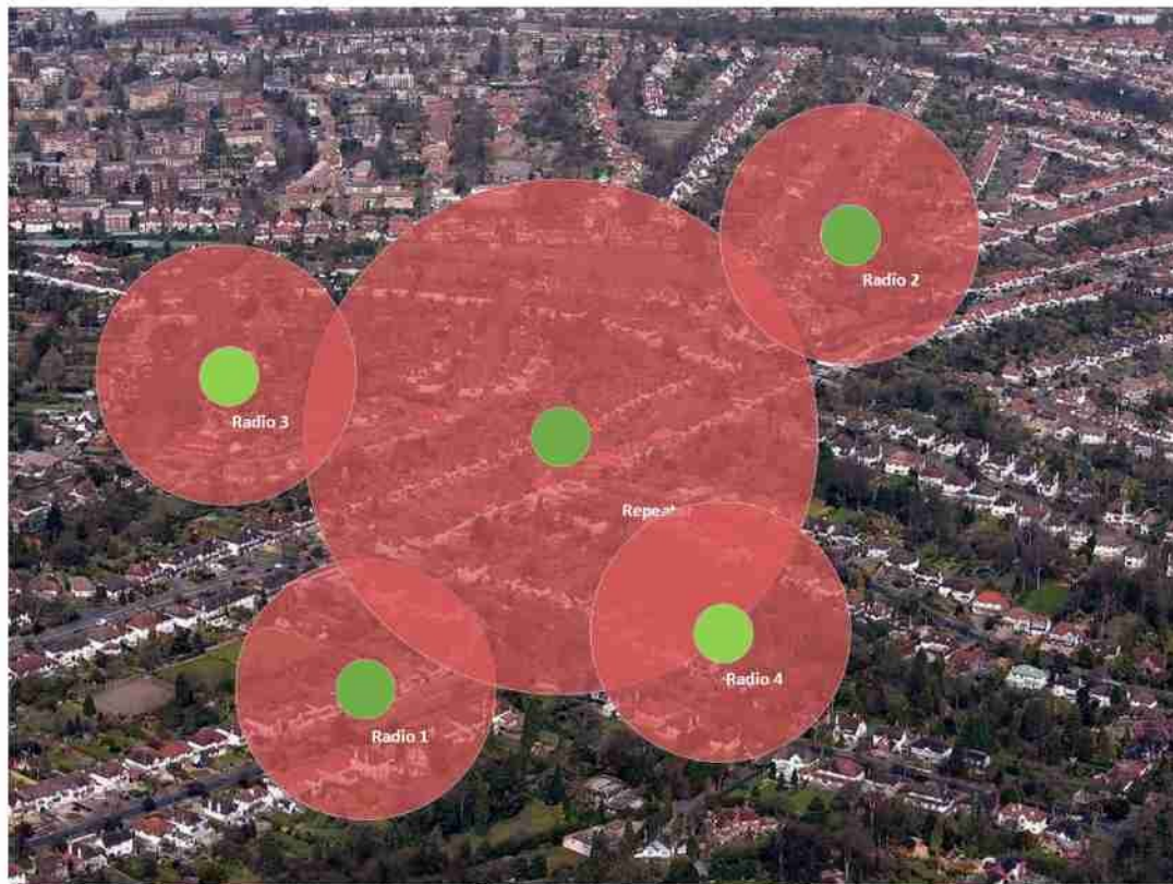
Figure 9 - Repeater positioned centrally between users
