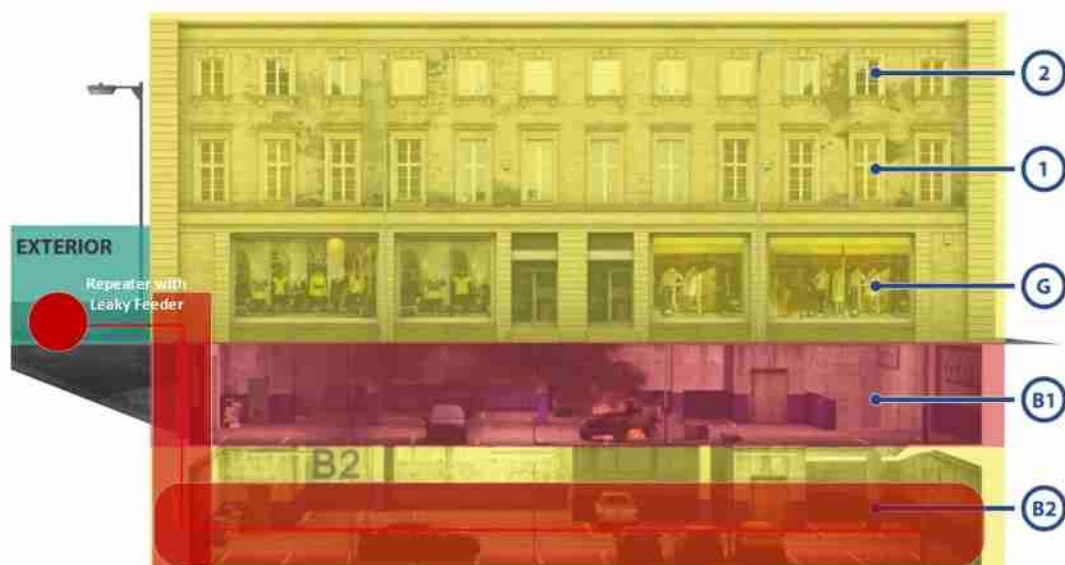
Figure 6 - Image showing leaky feeder deployment and coverage provided
