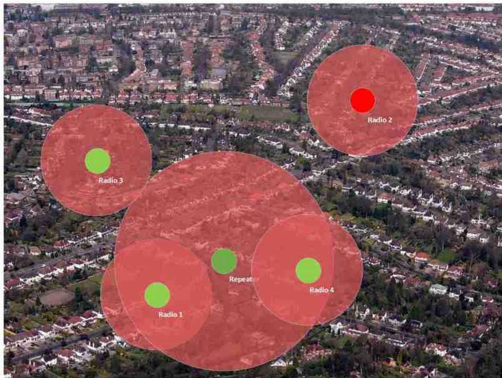
Figure 7 - Radio Coverage without a repeater
