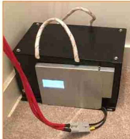
Figure 2 DIY domestic BESS
